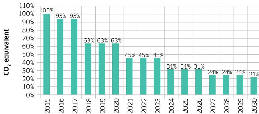
The CO<sub>2</sub> equivalent in the European Union is being incrementally lowered and restricted by the F-gas Regulation. (CO<sub>2</sub> equivalent = GWP value x filling volume)
